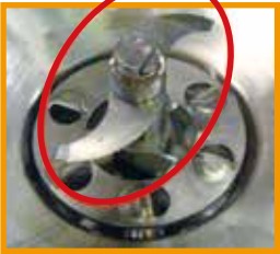
Chopper Blade work on (875rpm)
